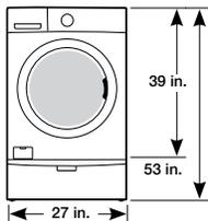
Required Dimensions for Installation With Stacking Kit
