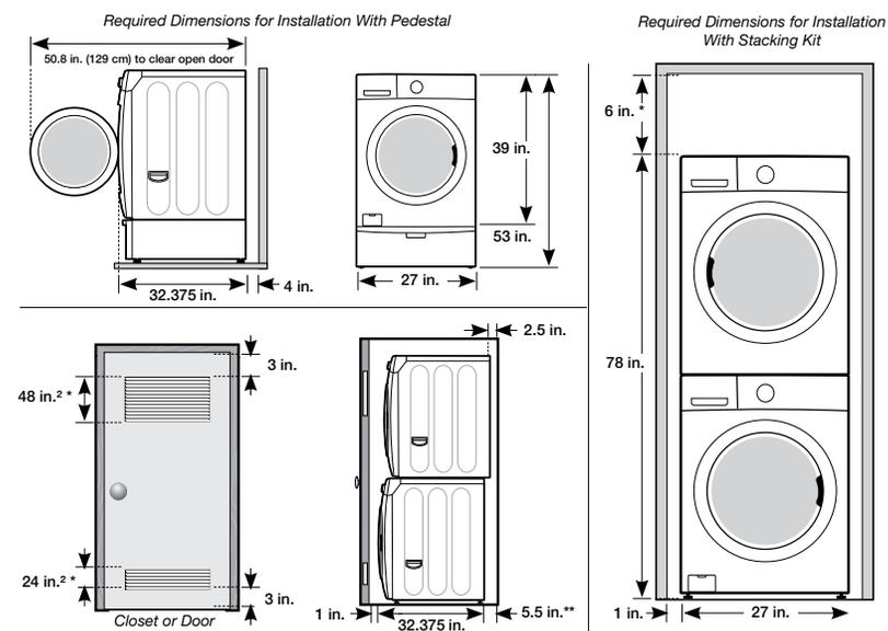
\* Required spacing    \*\* External exhaust elbow requires additional space.
