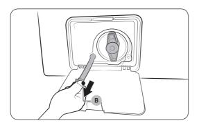
**3.** Put an empty, spacious container around the cover, and stretch the emergency drain tube to the container while holding the **tube cap (A)**.
