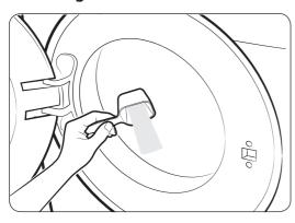
Oxygen boosters or color-safe bleach can increase washing performance. Make sure to add the oxygen booster or color-safe bleach after putting the laundry into the drum.
