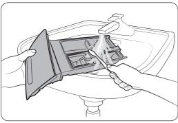
**3.** Clean the drawer components in flowing water using a soft brush.
