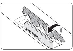
**2.** Open the adapter cover to reveal the protective cap of the adapter. Gently pull the cap to the right and lift up to remove.
