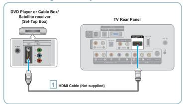
> Each DVD Player or Cable Box/Satellite receiver (Set-Top Box) has a different back panel configuration.
