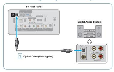
Connect an Optical Cable between the "DIGITAL AUDIO OUT (OPTICAL)" jacks on the TV and the Digital Audio Input jacks on the Digital Audio System.
