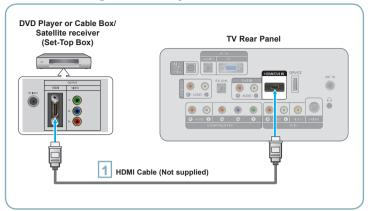
Each DVD Player or Cable Box/Satellite receiver (Set-Top Box) has a different back panel configuration. Connect an HDMI Cable between the HDMI/DVI IN jack on the TV and the HDMI jack on the DVD Player or Cable Box/Satellite receiver (Set-Top Box).
