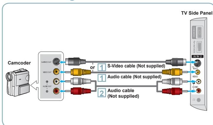
**1** Connect a Video Cable (or S-Video Cable) between the AV IN2 [VIDEO] (or S-VIDEO) jack on the TV and the VIDEO OUT jack on the camcorder.
