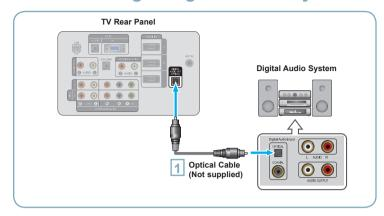
Connect an Optical Cable between the "DIGITAL AUDIO OUT (OPTICAL)" jacks on the TV and the Digital Audio Input jacks on the Digital Audio System.
