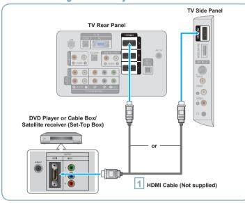
Connect an HDMI Cable between the HDMI IN (1, 2, 3 or 4) jack on the TV and the HDMI jack on the DVD Player or Cable Box/Satellite receiver (Set-Top Box).
