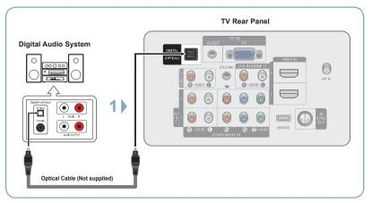
Connect an Optical Cable between the DIGITAL AUDIO OUT (OPTICAL) jacks on the TV and the Digital Audio Input (OPTICAL) jacks on the Digital Audio System.
