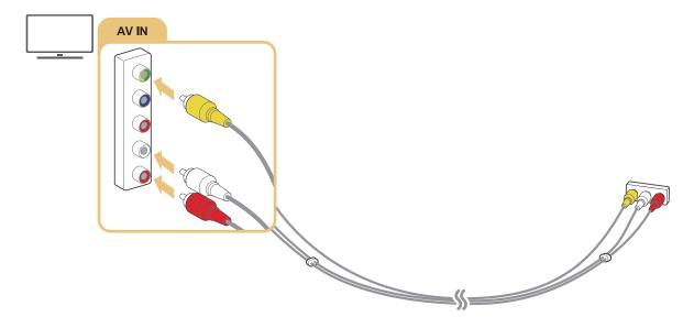
Connect AV (composite) equipment to AV In only. Do not connect to Component In.
