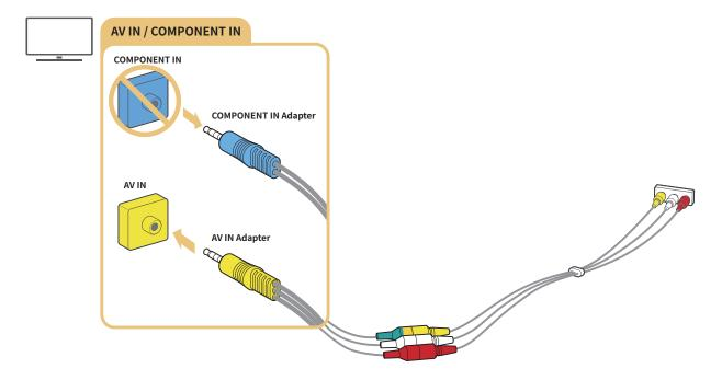
Connect AV (composite) equipment to AV In only. Do not connect to Component In.
