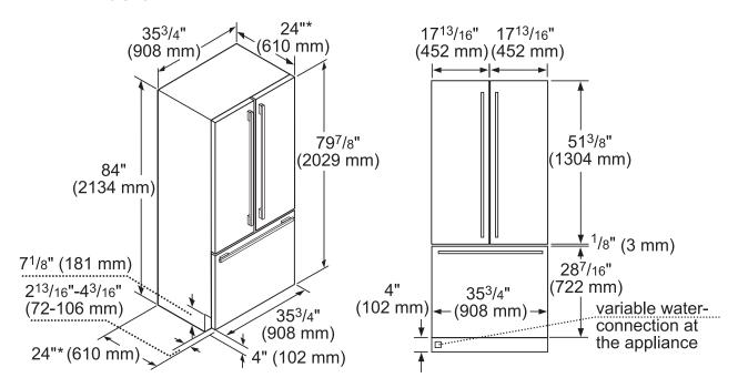
\*Excludes thickness of door panel. If standard panel with 3/4" thickness is mounted, total depth is 24 3/4".
