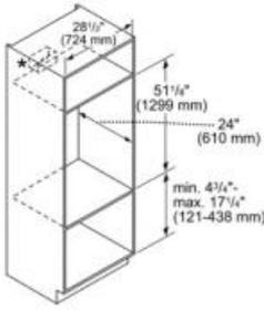
\* Junction box may be installed above, below or to the right of the unit, within reach of the power cable.
