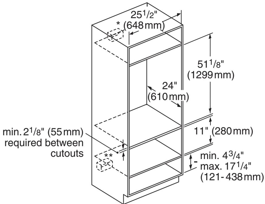
\* Wall oven junction box may be located above or right or left of the unit within reach of the power conduit.
