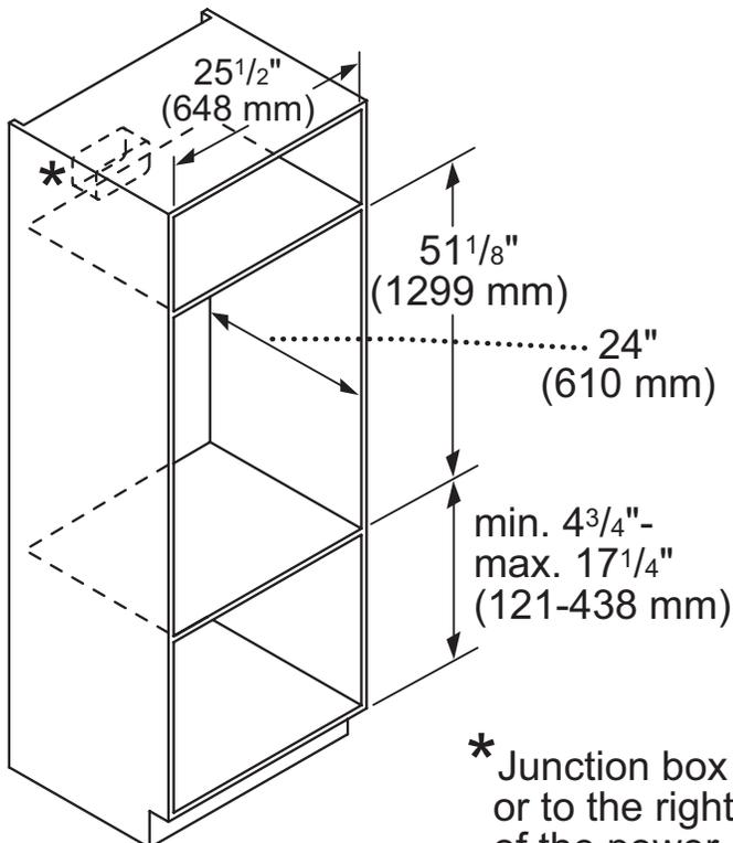
\* Junction box may be installed above, below, or to the right of the unit within range of the power cable.
