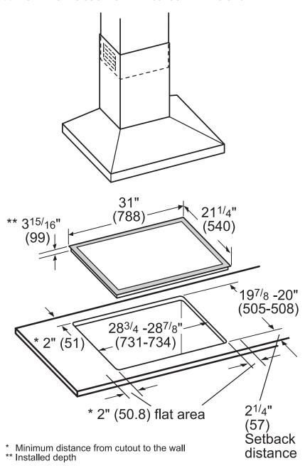
Measurements in inches (mm in brackets)
