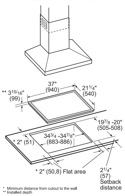
Measurements in inches (mm in brackets)
