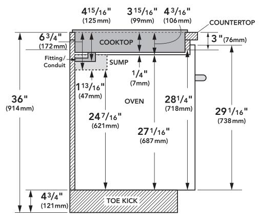
Note: Dimensions based on standard countertop height (36" with 43/4" toe kick including base plate).
