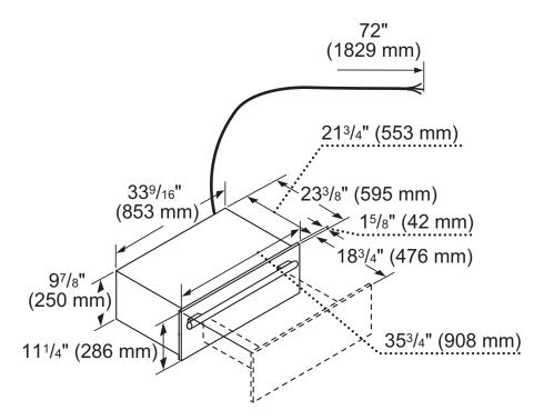
Note: 1 5/8" is the depth of the standard front panel (includes gasket). Dimension is not valid for custom panel product.
