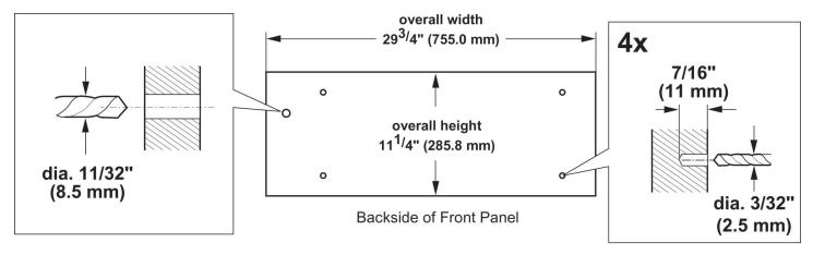
Hole for light wave guide Pilote holes
