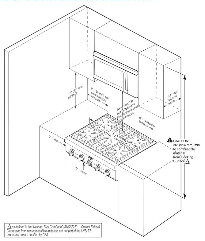
**NOTE:** A 36-inch minimum clearance is required between the top of the cooking surface and the bottom of an unprotected cabinet. A 30-inch clearance can be used when the bottom of the wood or metal cabinet is protected by not less than 1/4 inch of a flame retardant material covered with not less than No. 28 MSG sheet steel, 0.015 inch (0.4 mm) thick stainless steel, 0.024 inch (0.6 mm) aluminum, or 0.020 inch (0.5 mm) thick copper.
