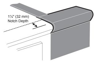
Front flush with cabinets; minimum of 24<sup>9</sup>/16<sup>"</sup> (624 mm) cabinet depth required.
