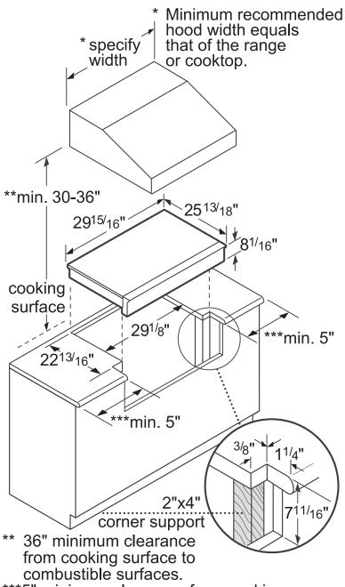
\*\*\*5" minimum clearance from cooking surface to combustible side wall.
