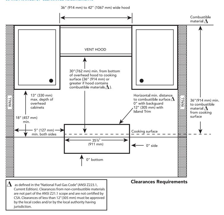
**NOTE:** A 36-inch minimum clearance is required between the top of the cooking surface and the bottom of an unprotected cabinet. A 30-inch clearance can be used when the bottom of the wood or metal cabinet is protected by not less than 1/4 inch of a flame retardant material covered with not less than No. 28 MSG sheet steel, 0.015 inch (0.4 mm) thick stainless steel, 0.024 inch (0.6 mm) aluminum, or 0.020 inch (0.5 mm) thick copper.
