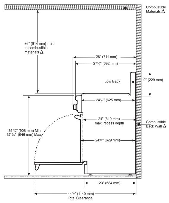
$\Lambda$  As defined in the "National Fuel Gas Code" (ANSI Z223.1, Current Edition). Clearances from non-combustible materials are not part of the ANSI Z21.1 scope and are not certified by CSA. Clearances of less than 12" (305 mm) must be approved by the local codes and/or by the local authority having jurisdiction.
