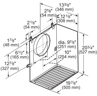
measurements in inches and mm
