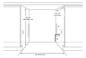
A: Recommended area for installation of power connection – a 2 ½" (63 mm) diameter hole is recommended 3: Location of power cord – approximately 15" (381 mm) from base of appliance
