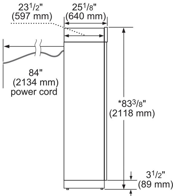
The depth from the front of the top grille to the back of the refrigerator cabinet is  $25\frac{1}{8}$ " (638 mm).
