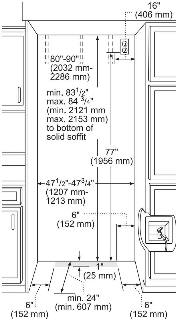
To avoid tipping during use, the solid soffit must be within 1" (25 mm) maximum above the refrigerator. If the solid soffit is higher than 1" (25 mm) or one is not available, then the refrigerator must be braced.
