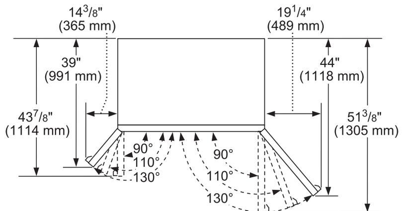
The location must permit both doors to open to a minimum of  $90^\circ$ . Allow  $4\frac{1}{2}$ " (114 mm) minimum space between the side of the refrigerator and a corner wall.
