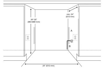
A: Recommended area for installation of power connection – a 2 1/2" (63 mm) diameter hole is recommended 3: Location of power cord – approximately 15" (381 mm) from base of appliance
