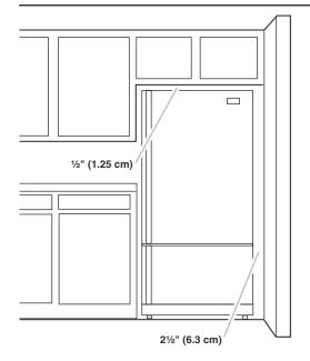
To ensure proper ventilation for your refrigerator, allow for a  $\frac{1}{2}$ " (1.25 cm) space at the top and behind the refrigerator. If your refrigerator has an ice maker, allow extra space at the back for the water line connections. When installing your refrigerator next to a fixed wall, leave  $2\frac{1}{2}$ " (6.3 cm) minimum on the hinge side (some models require more) to allow for the door to swing open.
