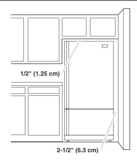
To ensure proper ventilation for your refrigerator, allow for 1/2" (1.25 cm) space at the top and behind the refrigerator. If your refrigerator has an ice maker, allow extra space at the back for the water connections. When installing your refrigerator next to a fixed wall, leave 2-1/2" (6.3 cm) minimum on the hinge side (some models require more) to allow for the door to swing open.
