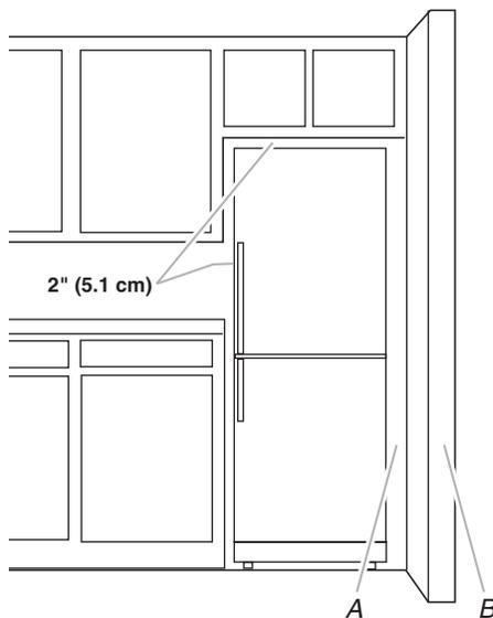
**Ventilation:** This refrigerator is designed for indoor, household use only. To ensure proper ventilation, allow for 2" (5 cm) of space between the top of the refrigerator and overhead cabinets and between the back of the refrigerator and the wall. If your refrigerator has an ice maker, allow extra space at the back for the water line connections. Keep the refrigerator ventilation openings clear.
