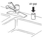
Make sure to use an air gap if the drain hose is connected to house plumbing lower than 20" (50.8 cm) above subfloor or floor.
