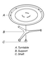
The turntable can rotate in either direction to help cook food more evenly. For best cooking results, do not operate the microwave oven without having the turntable in place. See "Assistance or Service" to reorder any of the parts.
