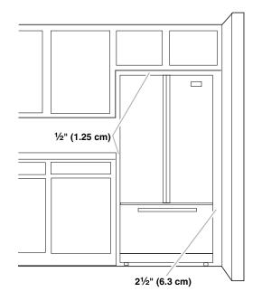
To ensure proper ventilation for your refrigerator, allow for  $\frac{1}{2}$ " (1.25 cm) space on each side and at the top. Allow at least 1" (2.54 cm) between the back of the cabinet and the wall. If your refrigerator has an ice maker, allow extra space at the back for the water connections. When installing your refrigerator next to a fixed wall, leave  $2\frac{1}{2}$ " (6.3 cm) minimum on each side (some models require more) to allow for the door to swing open.
