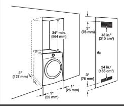
For closet installation, with a door, the minimum ventilation openings in the top and bottom of the door are required. Louvered doors with equivalent air ventilation openings are acceptable.
