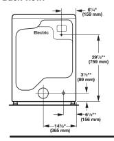
NOTE: Most installations require a minimum of 5" (127 mm) clearance behind dryer for exhaust vent with elbow. See "Venting Requirements."
