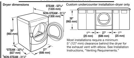
For closet installation, with a door, the minimum ventilation openings in the top and bottom of the door are required. Louvered doors with equivalent air ventilation openings are acceptable.
