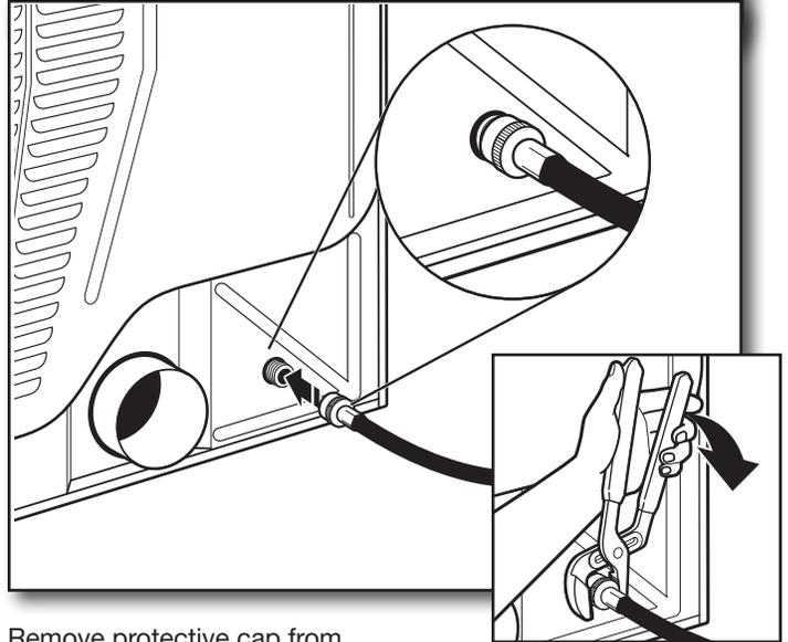
Remove protective cap from water inlet valve. Attach other end of long hose to fill valve at bottom of dryer back panel. Screw on coupling by hand until it is seated on fill valve connector. Using pliers, tighten the couplings an additional two-thirds turn.
