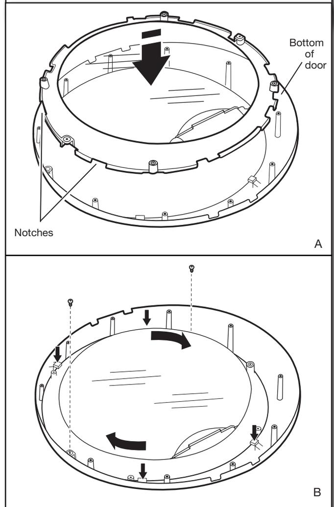
With the edge with 2 notches at the top, align the notches on the outer window assembly with the tabs on the trim ring and lower into place as shown in figure A. Rotate the outer window assembly counterclockwise to lock tabs into place (figure B). Using a Phillips screwdriver, secure with 2 screws removed earlier.
