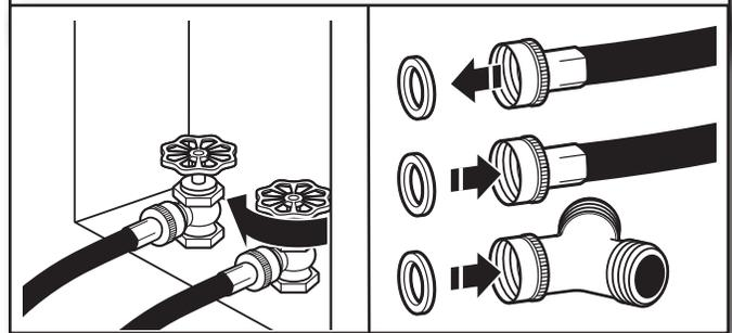
Turn cold water faucet off and remove washer inlet hose.
