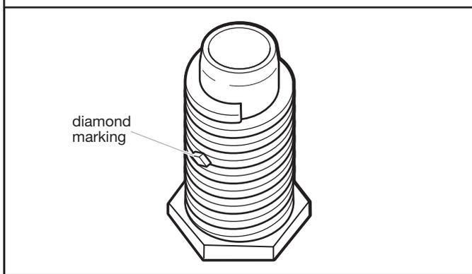
Examine leveling legs, find diamond marking. Screw legs into leg holes by hand, use a wrench to finish turning legs until diamond marking is no longer visible.
