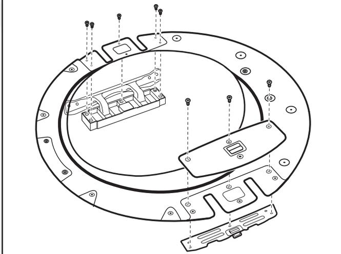
Using a Torx® † T25 screwdriver, reinstall the latch plate, latch backing plate, and hinge assembly on the opposite sides from which they were removed.
