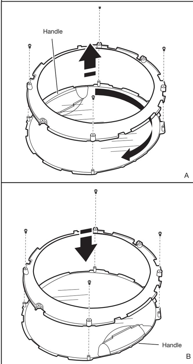
Using a Phillips screwdriver, remove the 4 screws from the outer window retainer and lift off the trim ring off the window (A). Rotate trim ring 180° and secure with the 4 screws removed earlier (B).
