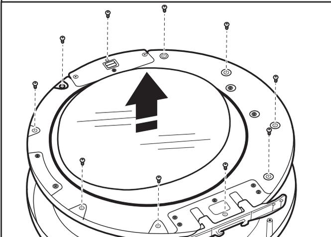
Position the door with the inside of the door facing up. Using a Phillips screwdriver, remove the 10 screws securing the inner door to the outer door. Lift off the inner door and set aside.
