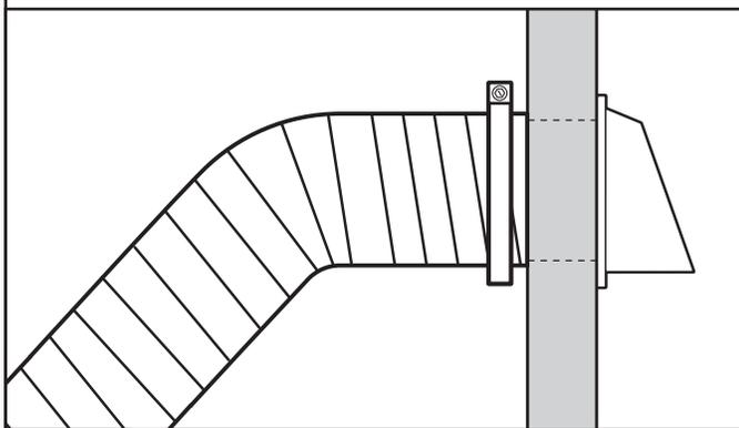
Vent must fit over the exhaust hood. Secure vent to exhaust hood with 4" (102 mm) clamp. Run vent to dryer location using straightest path possible. Avoid 90° turns. Use clamps to seal all joints. Do not use duct tape, screws, or other fastening devices that extend into interior of vent to secure vent, because they can catch lint.
