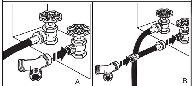
If space permits, attach the female end of the "Y" connector to the cold water faucet. See figure A.
