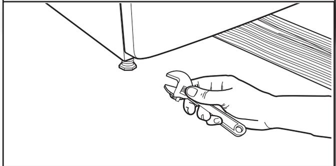
If dryer is not level, prop up using a wood block, use wrench to adjust legs up or down, and check again for levelness. Once dryer is level, make sure all four legs are snug against the floor and the dryer does not rock.
