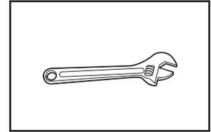
8" or 10" adjustable wrench (for gas connections)
