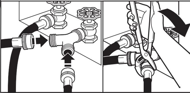
One end of the long hose has a wire mesh strainer inside the coupling. Attach this end to the “Y” connector. Attach washer cold inlet hose to other side of “Y” connector. Screw on coupling by hand until it is seated on connector. Using pliers, tighten the couplings an additional two-thirds turn.
