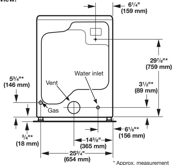
**NOTE:** Most installations require a minimum of 5" (127 mm) clearance behind dryer for exhaust vent with elbow. See "Venting Requirements".
