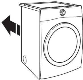
Move dryer to final location, taking care not to crush or kink vent or flexible gas line.
