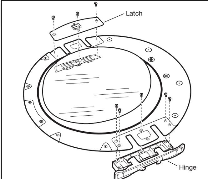
Using a Torx® † T25 screwdriver, remove the 3 Torx screws securing the latch plate and latch backing plate and the 5 screws holding the hinge assembly in place.
