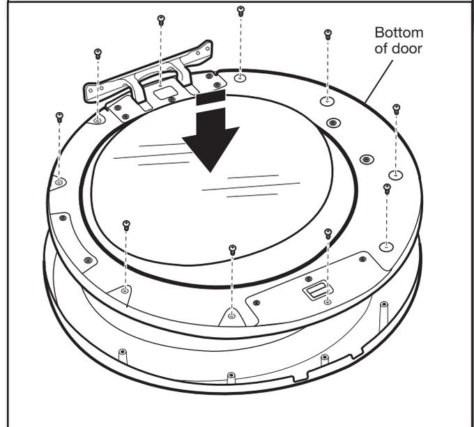
Position the door with the inside of the door facing up. Reinstall the 10 screws securing the inner door to the outer door.
