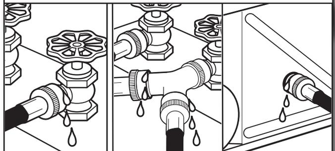
Check for leaks around “Y” connector, faucet, and hoses.
