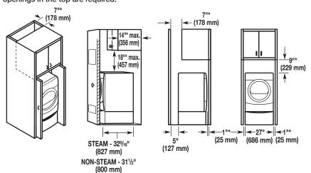
\*Required spacing \*\*For side or bottom venting, 2" (51 mm) spacing is allowed.
