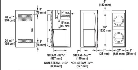
For cabinet installation, with a door, the minimum ventilation openings in the top are required.
