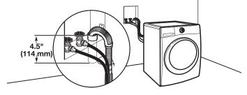
See requirements for floor standpipe drain system.
