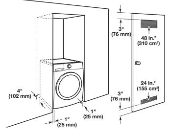
Recessed or closet installation - stacked washer and dryer
