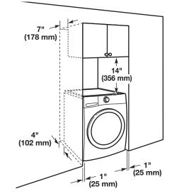
All dimensions show recommended spacing allowed, except for closet door ventilation openings which are the minimum required. For each arrangement, consider allowing more space for ease of
