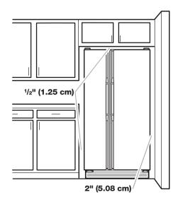
Normal minimum cabinet cut-out width required for product installation is 36" (91.4 cm). However, if the product is placed against an extended wall and the ability to remove the crisper pans is desired, an additional 18" (45.7 cm) of cabinet width is required, so a total cabinet opening width of 54" (137.2 cm) is recommended.
