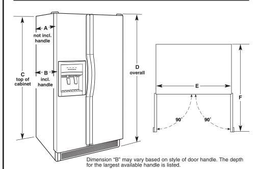
Dimensions "C" and "D" include the leveling legs extended to the minimum height of  $\frac{1}{4}$ " (6.35 mm) below the refrigerator. When leveling legs are fully extended to 1" (2.54 cm), add  $\frac{3}{4}$ " (19.05 mm).
