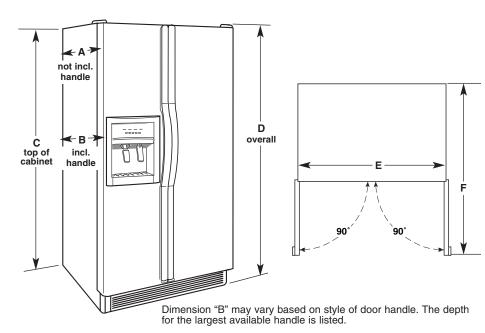
Dimensions "C" and "D" include the leveling legs extended to the minimum height of  $\frac{1}{2}$ " (6.35 mm) below the refrigerator. When leveling legs are fully extended to 1" (2.54 cm), add  $\frac{3}{2}$ " (19.05 mm).
