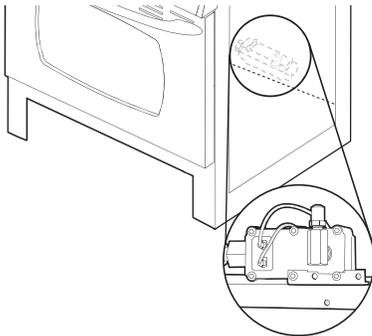
2. Using an adjustable wrench, turn the Number .0512 LP gas oven bake burner orifice hood counterclockwise to remove.
