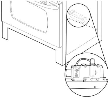
2. Using an adjustable wrench, turn the Number 49 Natural gas oven bake burner orifice hood counterclockwise to remove.
