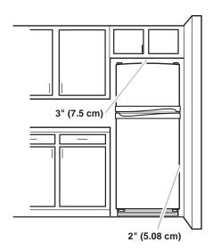
To ensure proper ventilation for your refrigerator, allow for a 1/2 in. (12.7 mm) space on each side. Allow 3 in. (7.5 cm) of space between overhead cabinets and refrigerator top. Allow at least 1 in. (2.5 cm) between back of cabinet and the wall. If your refrigerator has an ice maker, make sure you leave some extra space at the back for the water lin connections.
