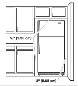
To ensure proper ventilation for your refrigerator, allow for a  $\chi'''$  (1.25 cm) space on each side and at the top. Allow at least 1" (2.54 cm) between back of cabinet and the wall. If your refrigerator has an ice maker, make sure you leave some extra space at the back for the water line connections.
