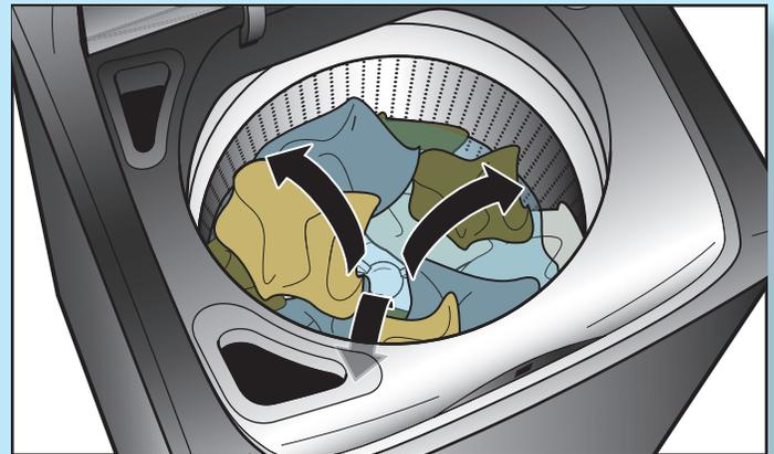
The impeller moves the load through the water while using less water and energy compared to a traditional agitator-style washer.
