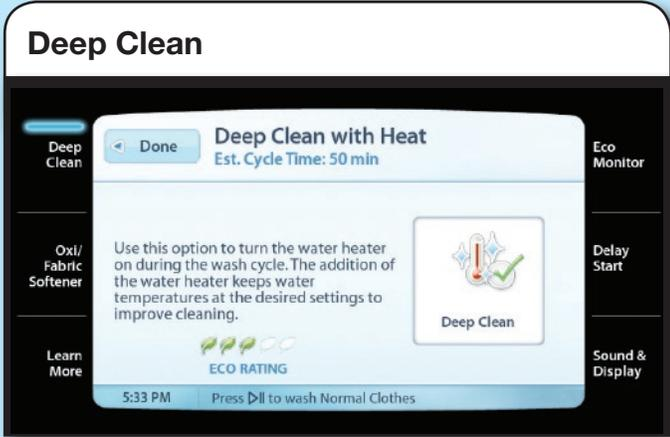
Touch to activate the Deep Clean with Heat option. This option adds additional soak and agitation time to help remove tough stains. An integrated heater helps to maintain optimal wash temperatures.
