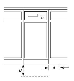
A. Leave 6" (15.2 cm) of clearance space to the right side of the compactor in order to remove the compactor bags.
