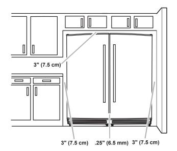
Allow at least 3 in. (7.5 cm) of air space at the top and on both sides of the appliances with 1/4 in. (6.5 mm) between the freezer and refrigerator. Allow 1 in. (2.5 cm) between the back of the appliances and the wall. If the appliances are to be against a side wall, leave extra space on the hinge sides so the door can open wider.
