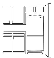
**IMPORTANT:** Do not install the freezer near an oven, radiator, or other heat source, nor in a location where the temperature will fall below 40°F (5°C).
