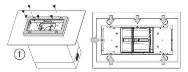
B - Take out the spacer, by removing the (6) plus (4) metric screws and the bushes.
