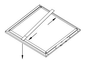
Secure charcoal filters to back side of baffle filters by two brackets for each filter
