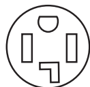
4-wire receptacle (14-30R)
