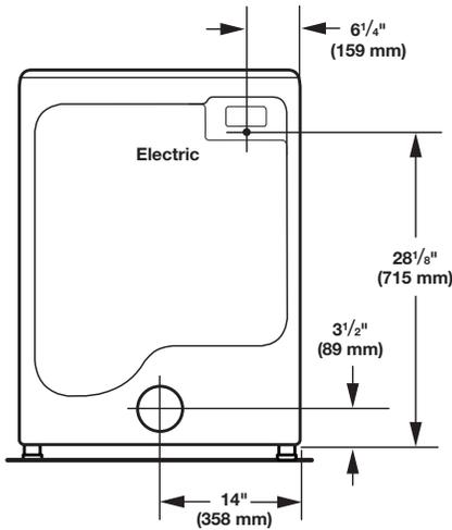
**NOTE:** Most installations require a minimum 5" (102 mm) clearance behind the dryer for the exhaust vent with elbow. See "Venting Requirements".
