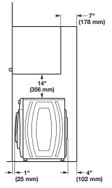
All dimensions show recommended spacing allowed, except for closet door ventilation openings which are the minimum required.
